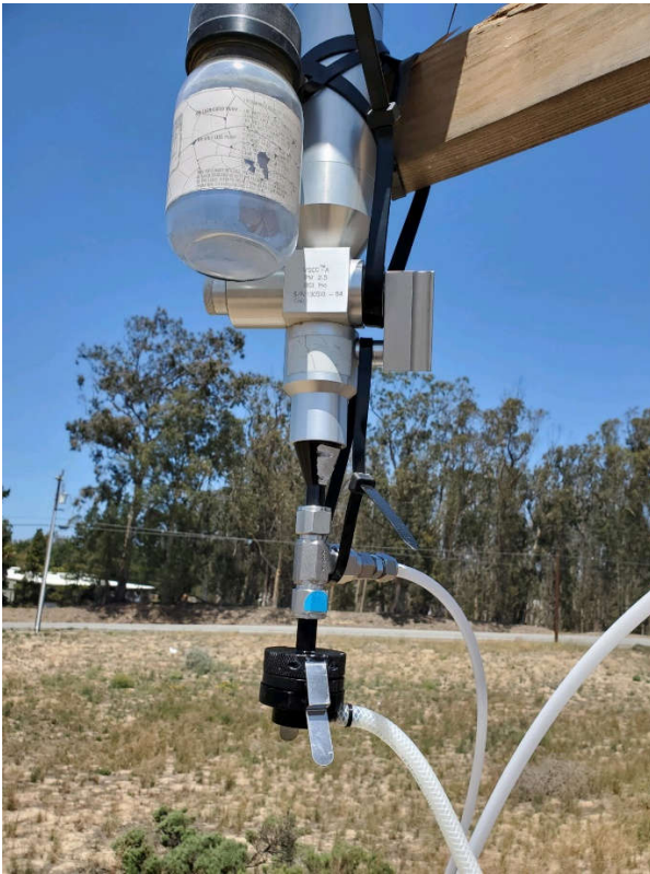
Figure 1: Scripps's PM_{2.5} sampling setup for 2021. Note the T fitting and bypass flow between the VSCC and the sample holder.
